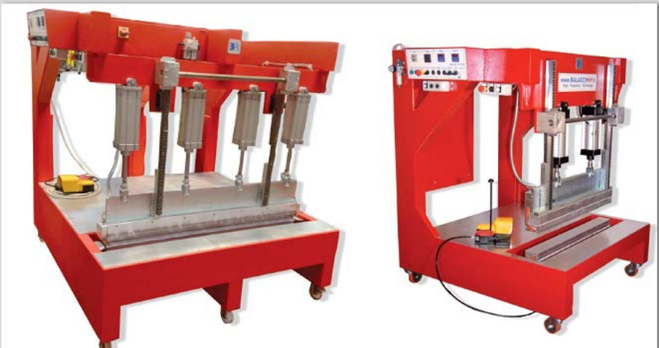
The BR10 PTFE welders are available in various size and for various purposes. This machine operates in two-step positioning mode that enables the precise placing of material and straight welding seam effectively avoiding the accidental seaming. Welding rod is usually 100x1000mm, but it could be upgraded according to client's demands. Special engraved electrodes are also available.
